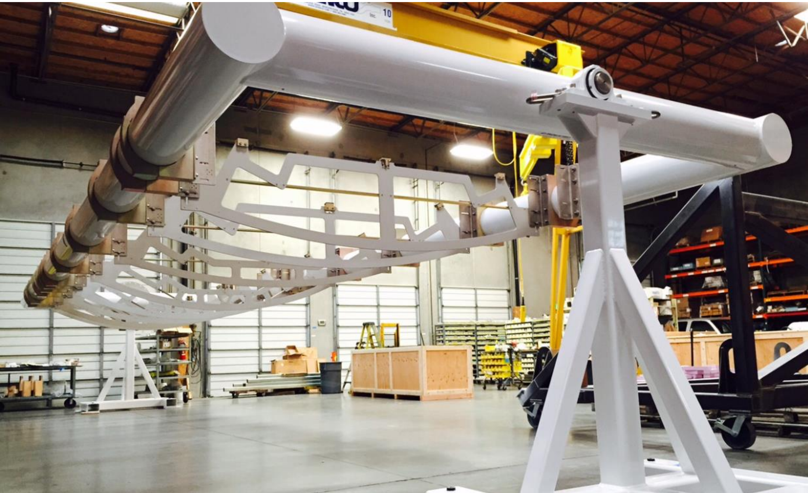
Flotron Rotation Fixture and Payload Interface Hardware Support NG JWST Composite Spacecraft Structure Assembly
