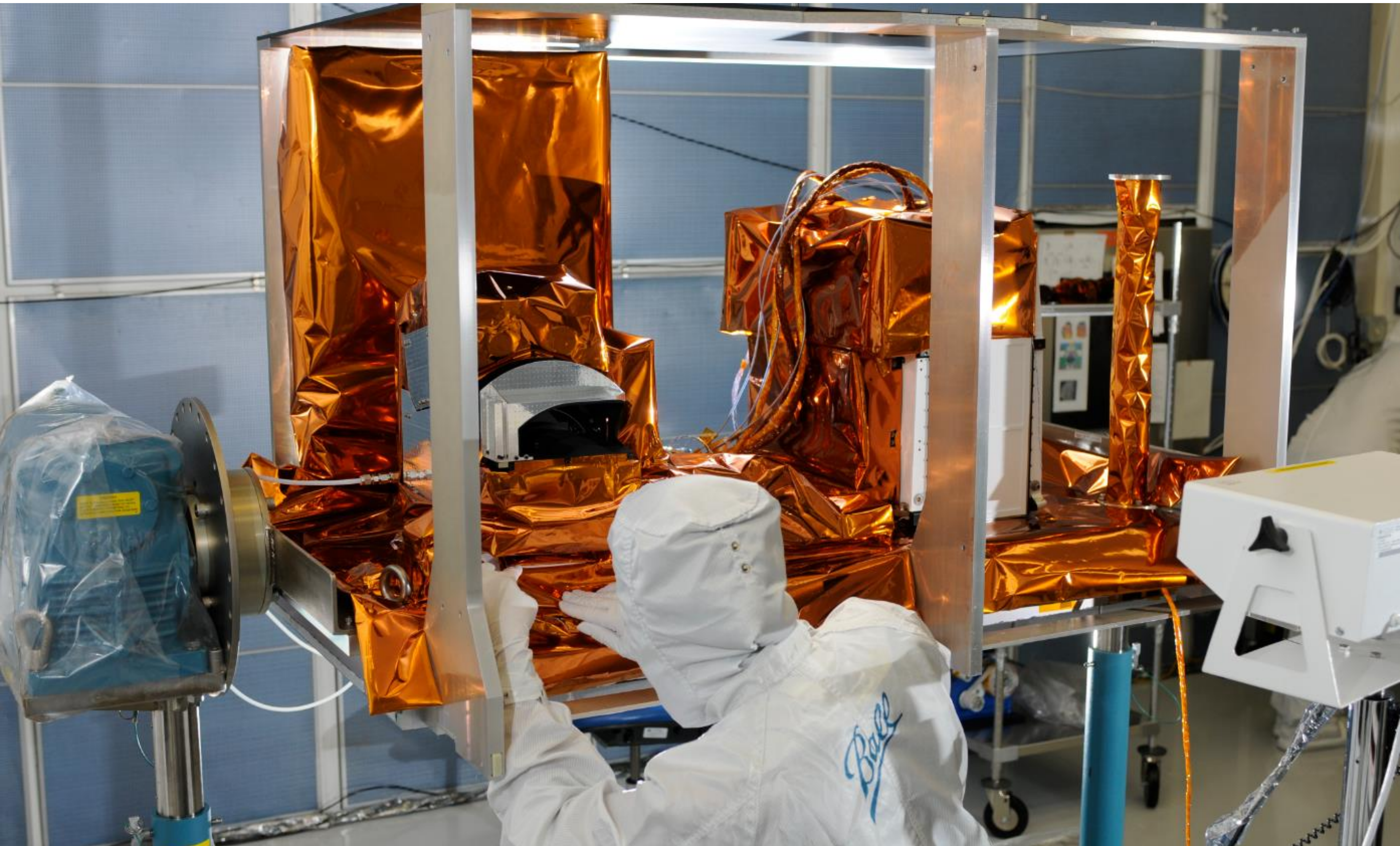
Flotron Rotation Fixture provides BATC technicians ergonomic access during AI&T of the Ozone Mapping and Profiler Suite (OMPS)
