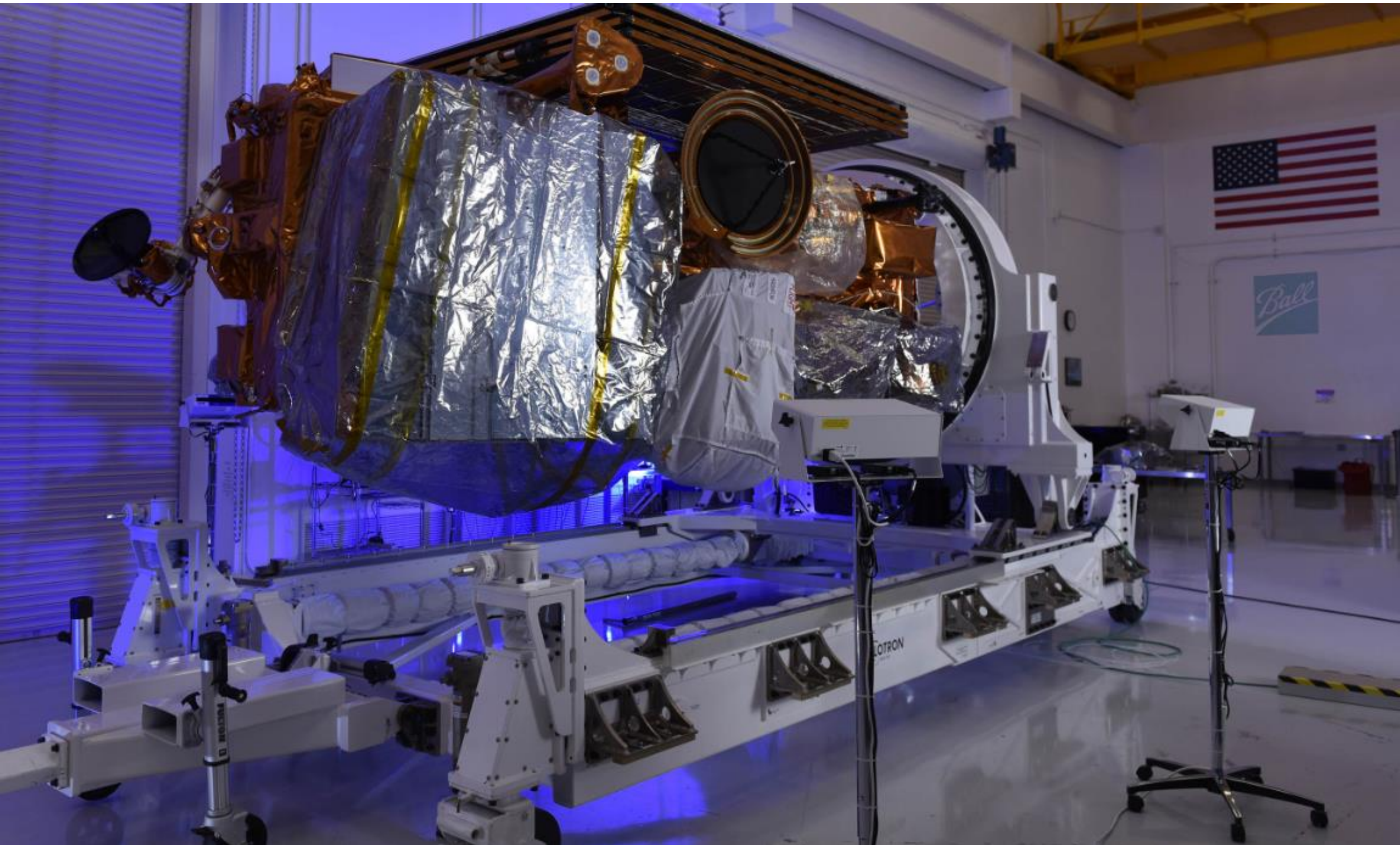
Flotron Satellite Positioner transports and Upends JPSS-1 NASA/NOAA next generation Weather Satellite.
