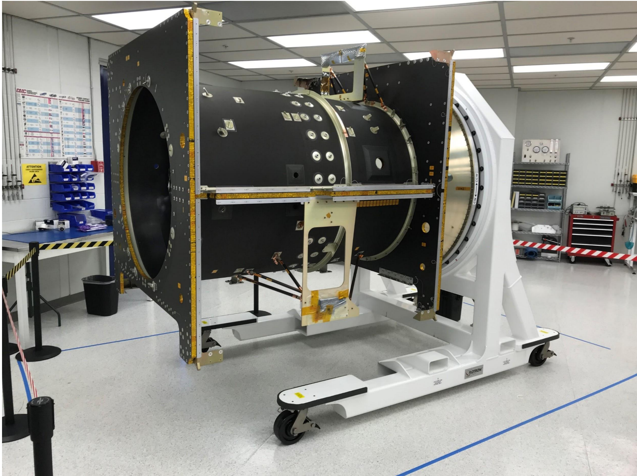
Flotron Satellite Integration Fixture supporting a spacecraft structure for a scientific mission.
