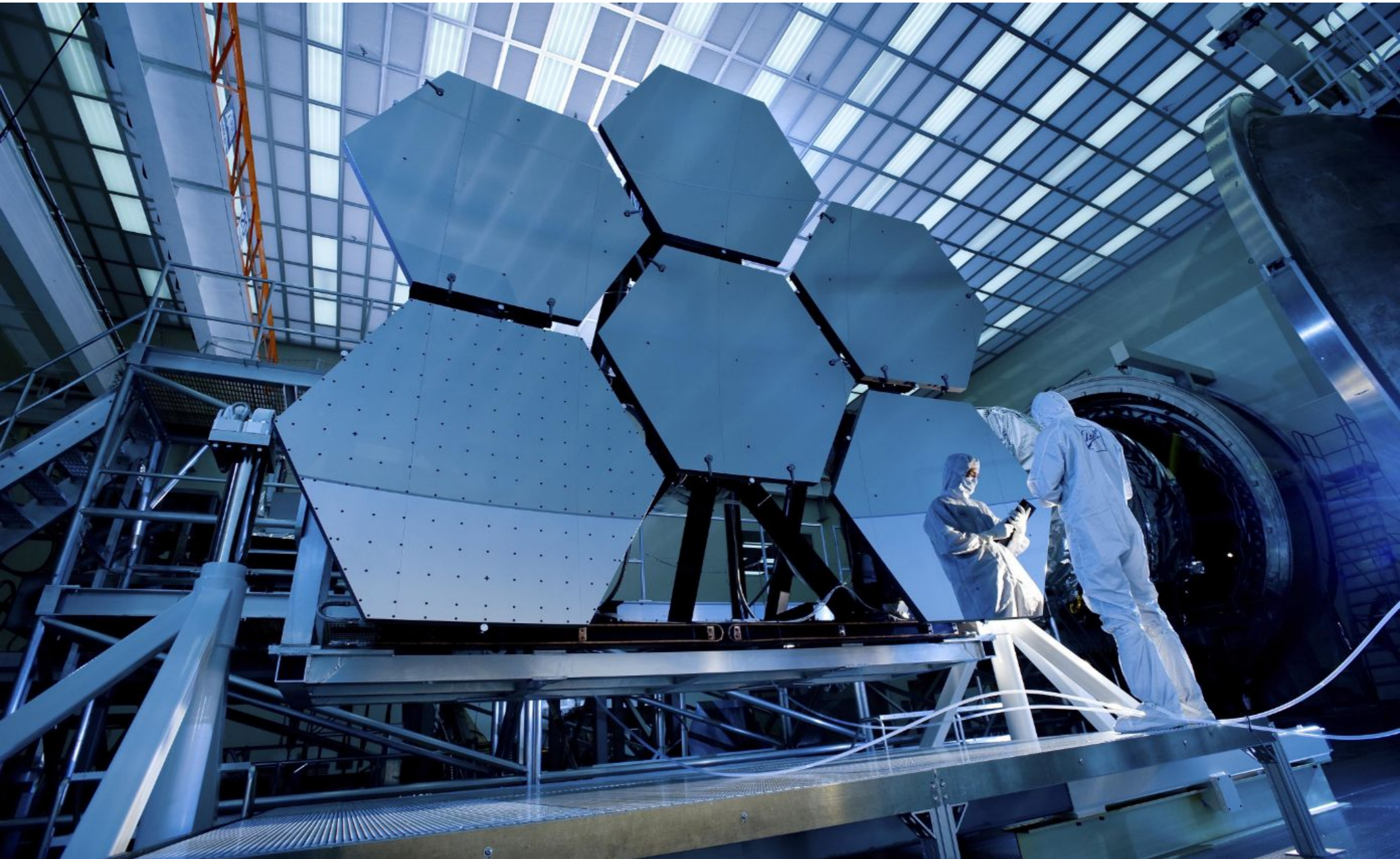
Flotron Rotation Fixture supports six BATC beryllium mirror segments between a series of cryogenic tests.
