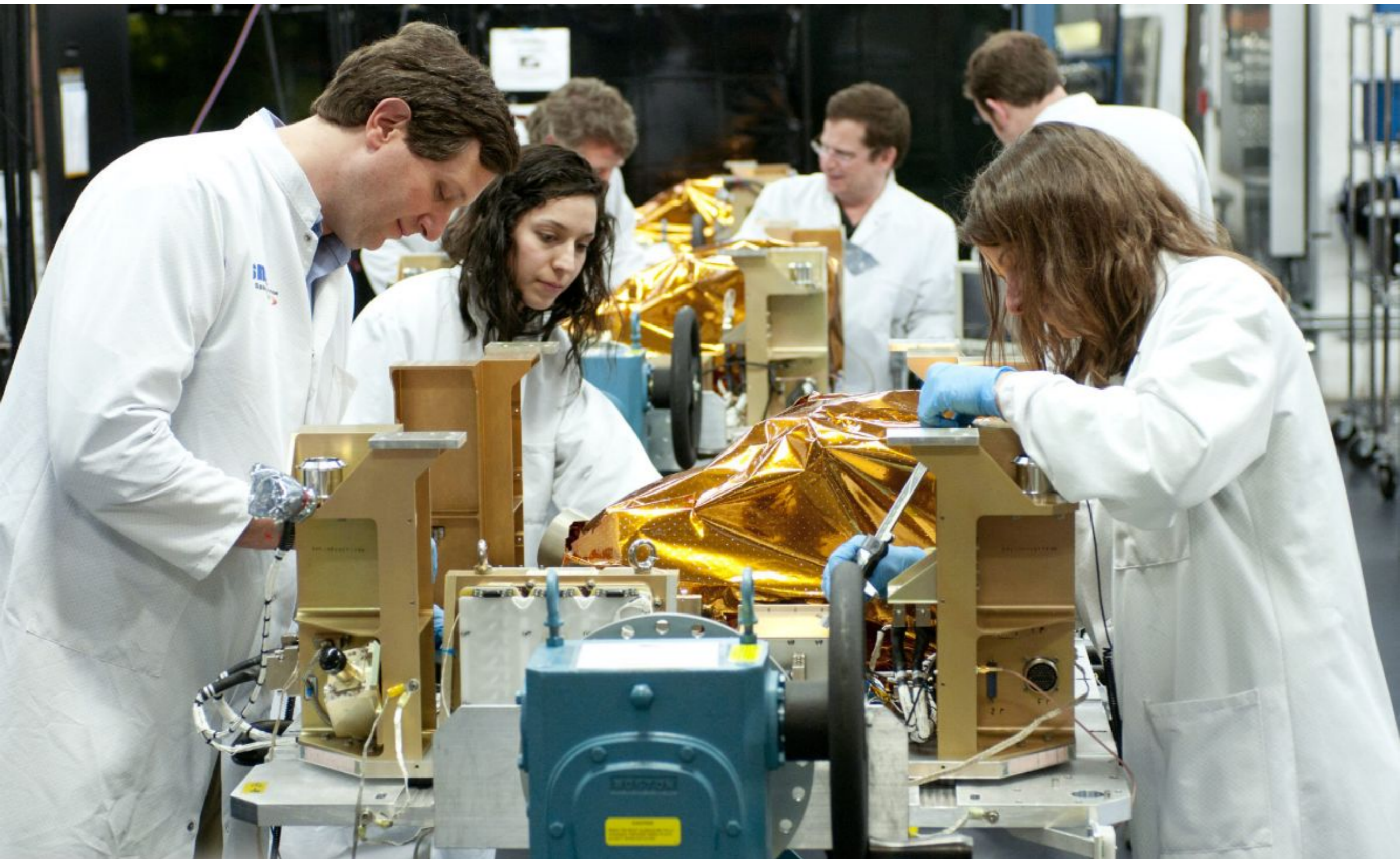
Flotron Rotation Fixture provides SNC technicians ergonomic access during AI&T of OG2 Satellites
