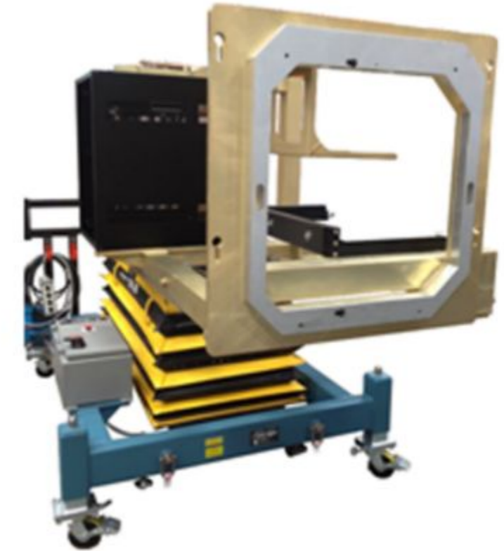
Cantilevered, Motorized Height Adjustment with Scissor Lift
