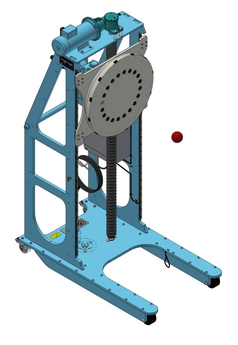
902:1 RATIO GEARING SYSTEM-HAND WHEEL IS REMOVABLE FOR USE OF DRILL DRIVE (3/8" SQ DRIVE SOCKET INCLUDED WITH FIXTURE) -600 LBS SIMULATION PAYLOAD COMBINED FIXTURE & PAYLOAD CG 57.00 MAX (SHOWN) 20 MIN **PUSH BAR** 5.05 GROUND CLEARANCE Ø3.00 X 2.00 WIDE POLYURETHANE **→** 16.74 CG → Ø3.00 X 1.50 WIDE NYLON WHEEL WHEEL FIXED AXLE SWIVEL CASTERS WITH BRAKE NO BRAKE NON-LOCKING LONGITUDINAL TIPOVER: 16.74 / 41.20 = .40G
