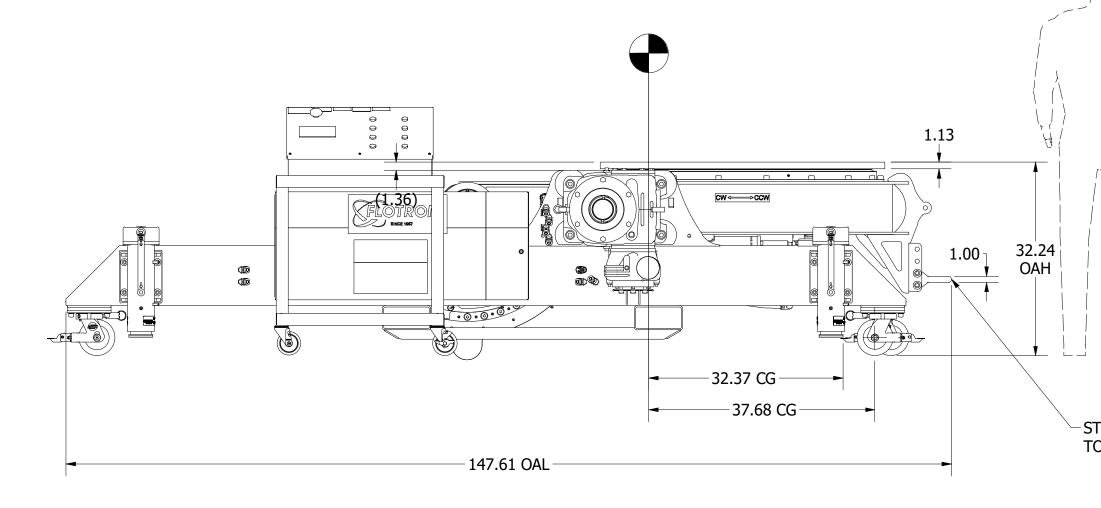
LONGITUDINAL STABILITY ON CASTERS WITH PAYLOAD VERTICAL: 31.53 / 48.80 = .64G LONGITUDINAL STABILITY ON JACKS WITH PAYLOAD VERTICAL: 36.84 / 54.73 = .67G LATERAL STABILITY ON CASTERS WITH PAYLOAD VERTICAL: 24.10 / 48.80 = .49G LATERAL STABILITY ON JACKS AT MAX STROKE WITH PAYLOAD VERTICAL: 33.80 / 54.73 = .61G
