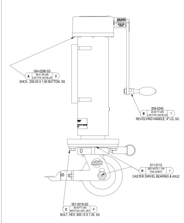
(BLANK) - LUBRICATE SCREW AND GEARS, WITH SYNCO SUPER LUBE GREASE (MMC #1353K1). LUBRICATE CASTER SWIVEL BEARING & AXLE WITH GENERAL PURPOSE BEARING GREASE.
